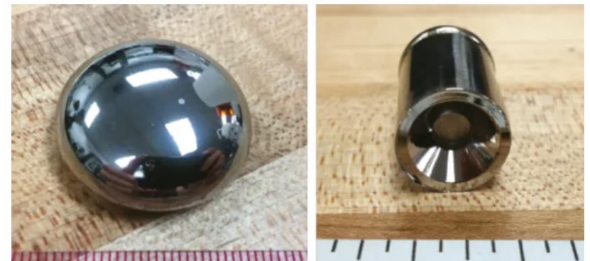
A 30-g ingot of the BMG Ti40Zr20Cu5Al5Be30 with a measured density of 4.76 g/cm 3
